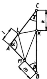
$$\left. \begin{aligned} F_{LAM} &= \frac{1}{2} l(c - m) \sin \alpha \\ F_{MBK} &= \frac{1}{2} m(a - k) \sin \beta \\ F_{KCL} &= \frac{1}{2} k(b - l) \sin \gamma \end{aligned} \right\} \quad (26)$$
