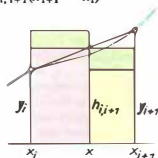
28.3-2 Zur Aitken-Interpolation; h_{i, i+1}(x_{i+1} - x_i) = y_i(x_{i+1} - x) + y_{i+1}(x - x_i)
