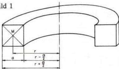
$$V = V_a - V_i = \pi r_a^2 a - \pi r_i^2 a = \pi a (r_a^2 - r_i^2)$$
