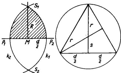
$$\begin{aligned} (r+s)^2 + \left(\frac{d}{2}\right)^2 &= d^2 \\ s^2 + \left(\frac{d}{2}\right)^2 &= r^2 \\ 2rs &= d^2 - 2r^2 \\ r^2s^2 &= \left(\frac{d^2}{2} - r^2\right)^2 \\ r^2\left(r^2 - \frac{d^2}{4}\right) &= \frac{d^4}{4} - r^2d^2 + r^4 \\ \frac{3}{4}r^2 &= \frac{d^2}{4} \\ r &= \frac{d}{3}\sqrt{3} \end{aligned}$$
