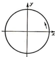
$$\begin{aligned}x &= a \cdot \sin t \\y &= a \cdot \sin\left(t - \frac{\pi}{2}\right) \\ \omega_1:\omega_2 &= 1:1\end{aligned}$$
