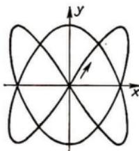
$$\begin{aligned}x &= a \cdot \sin 2t \\y &= a \cdot \sin 3t \\ \omega_1:\omega_2 &= 2:3\end{aligned}$$
