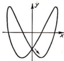
$$\begin{aligned}x &= a \cdot \sin t \\y &= a \cdot \sin\left(2t - \frac{\pi}{2}\right) \\ \omega_1:\omega_2 &= 1:2\end{aligned}$$
