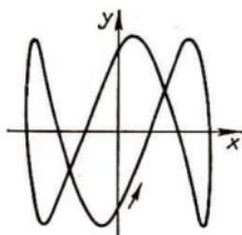
$$\begin{aligned}x &= a \cdot \sin t \\y &= a \cdot \sin\left(3t - \frac{\pi}{2}\right) \\ \omega_1:\omega_2 &= 1:3\end{aligned}$$
