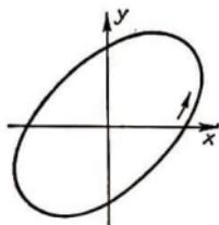
$$\begin{aligned}x &= a \cdot \sin t \\y &= a \cdot \sin\left(t - \frac{\pi}{3}\right) \\ \omega_1:\omega_2 &= 1:1\end{aligned}$$
