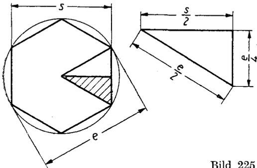
$$\begin{aligned} \left(\frac{s}{2}\right)^2 &= \left(\frac{e}{2}\right)^2 - \left(\frac{e}{4}\right)^2 \\ &= \frac{e^2}{4} - \frac{e^2}{16} = \frac{3}{16} e^2; \end{aligned}$$
