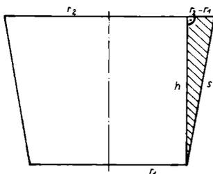
$$A_1 = \pi[(r_1 + r_2)\sqrt{h^2 + (r_2 - r_1)^2} + r_1^2]$$
