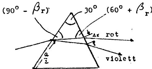
$$\Delta x = \frac{s}{2} \cdot \left| \frac{\sin (90^\circ - \beta_r)}{\sin (60^\circ + \beta_r)} - \frac{\sin (90^\circ - \beta_v)}{\sin (60^\circ + \beta_v)} \right|$$
