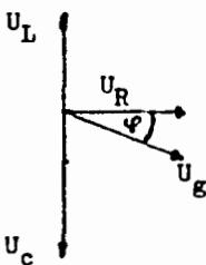
$$\begin{aligned} c) \quad \varphi &= \arctan (X_L - X_C)/R \\ &= 40^\circ \\ &===== \end{aligned}$$
